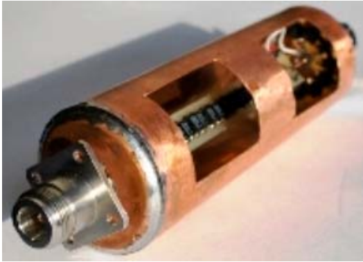
Fig. 2 A photograph of the internal part of a resistive divider
