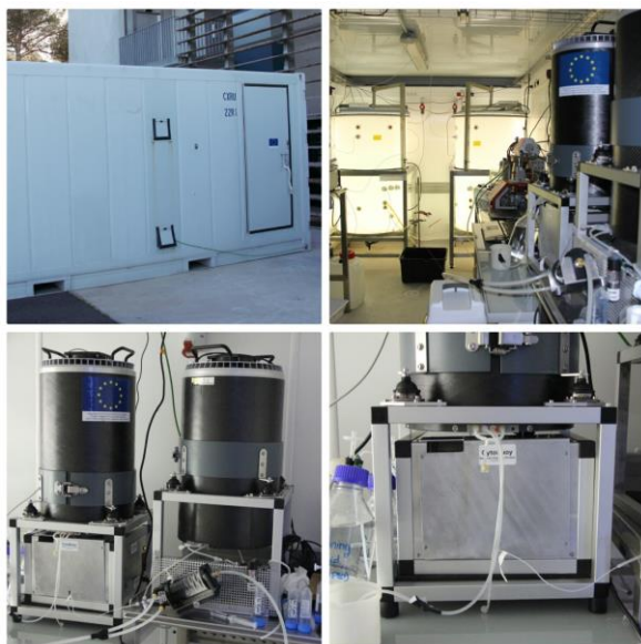
Fig. 1. Installation of Cytosenses in MIO experimental container
