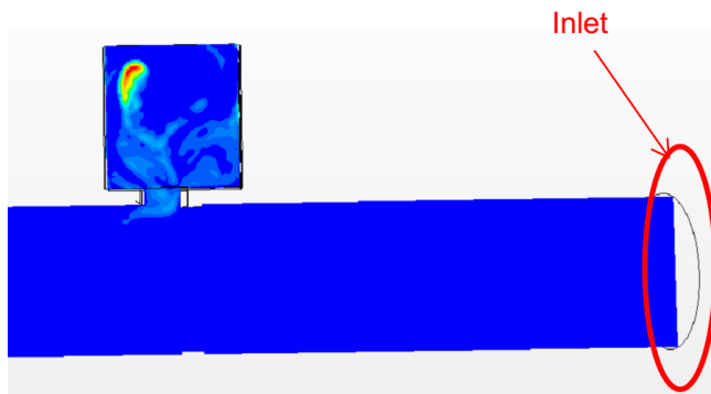
Fig.4 View of pressure chamber along the meter axis for shape B, showing minimal amount of air. Flow velocity u = 3 \text{ m/s}
