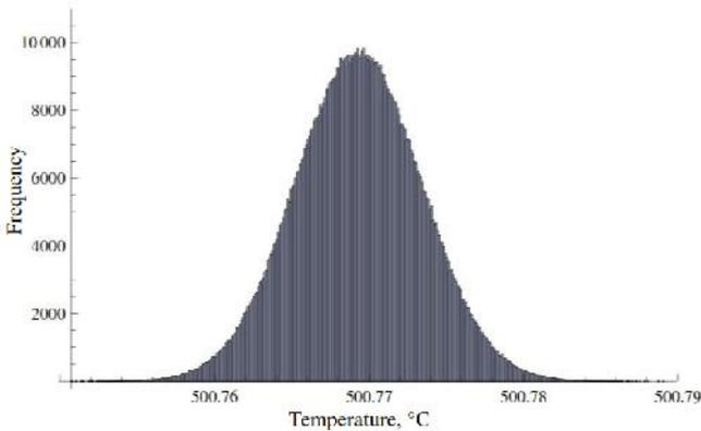
Fig. 3. The distribution of temperature determined by Monte Carlo method at 500 °C
