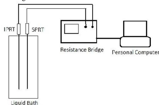
Fig. 1. Calibration setup.
