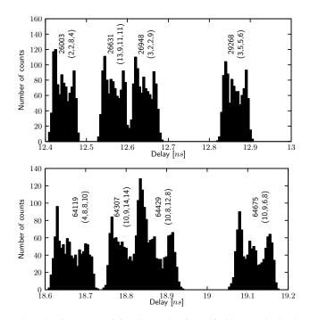
Fig. 15. Histograms of time-intervals of specified length obtained for eight different control-values. Control-values are placed in parenthesis with indexes above them.
