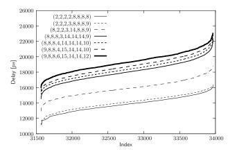
Fig. 11. DCDEs delay dependency from control-values. Control-values changes in such ranges that guarantee constant standard-deviation and variable average value.
