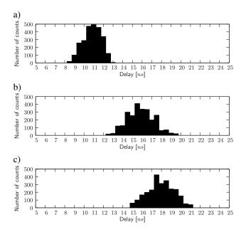
Fig. 16. Histograms of time-intervals of specified Gaussian distribution with constant standard-deviation. Control-values change in ranges (a) (2,2,2,2,5,5,5), (b) (5,5,5,5,8,8,8,8) and (c) (6,6,6,6,9,9,9,9)
