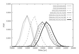
Fig. 13. Probability density functions of time-intervals obtained from serially connected digitally-controlled-delay-elements that characteristics have been presented in Fig. 11
