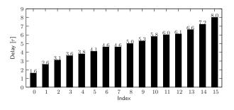
Fig. 3. The characteristic of two serially connected digitally-controlled-delay-elements.
