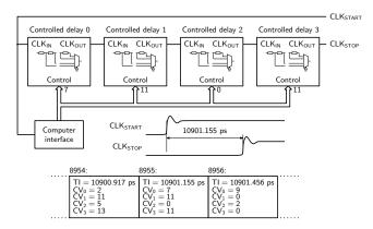
Fig. 5. Specified length time-interval generator.
