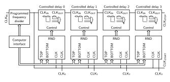
Fig. 7. Specified Gaussian distribution time-interval generator.
