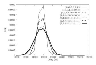
Fig. 14. Probability density functions of time-intervals obtained from serially connected digitally-controlled-delay-elements that characteristics have been presented in Fig. 12
