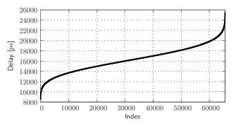
Fig. 9. DCDEs delay dependency from control-values index (control-values were changing in full range).
