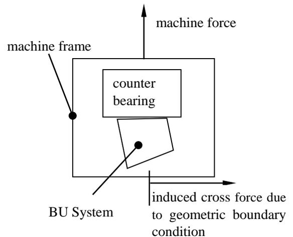
Figure 7.6: geometrical boundary condition in hydraulic machines
