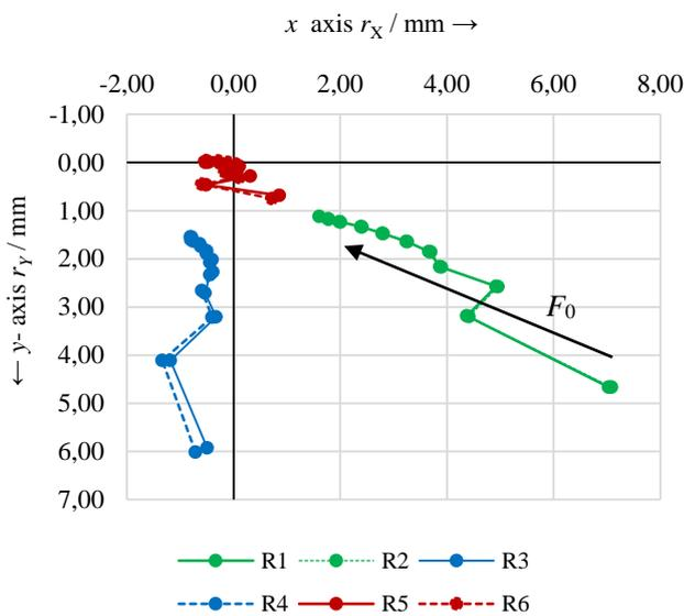
Figure 7.4: movement of the load center in a force standard machine
