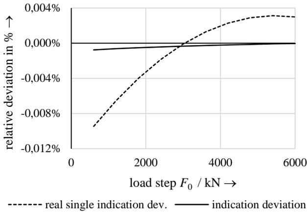
Figure 7.1 indication deviations performing BU system calibration
