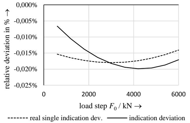
Figure 7.2: indication deviations performing intercomparison
