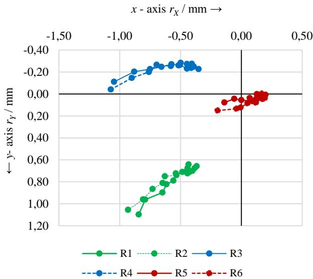
Figure 7.7: load center in a hydraulic machine with spherical cap
