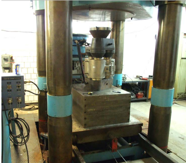
Fig. 1. 30 MN calibration facility with mounted 15 MN BU system during preload test in Odessa
