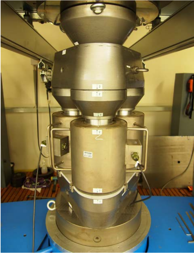
Fig. 7. Photo of the 15 MN BU system mounted in PTB's 16.5 MN FSM
