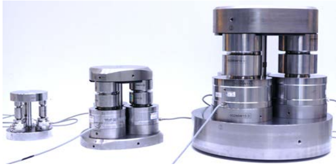
Fig. 6. 3 x 20 kN, 3 x 1 MN and 3 x 2 MN BUS system of same type
