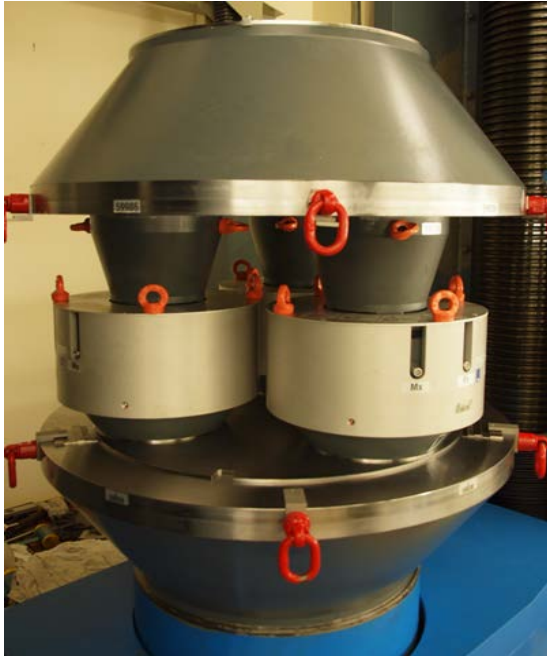
Fig. 3. Three 10 MN transducers mounted with the adaptation parts for five transducers to achieve a higher stiffness in comparison with the smaller parts of the 30 MN system (Fig. 2)
