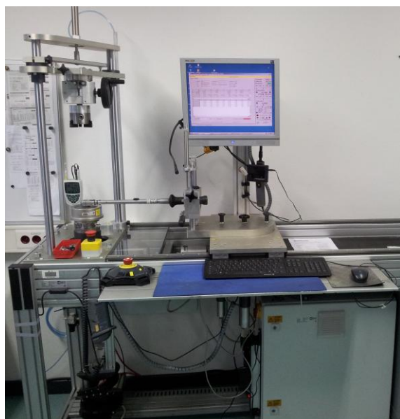
Fig. 2. Torque wrench calibration device (by courtesy of CEH).
