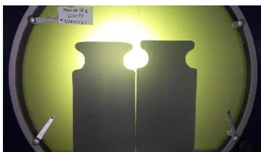
Fig. 3. Projection of two weights with different trademark and same nominal value (10 g) and OIML R 111-1 classification (E 2 ).
