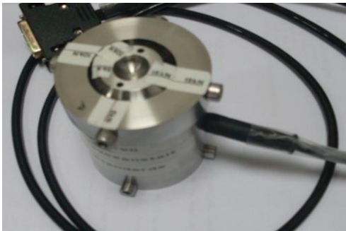
Fig. 8. Manufactured multi-capacity load cell without loading plate
