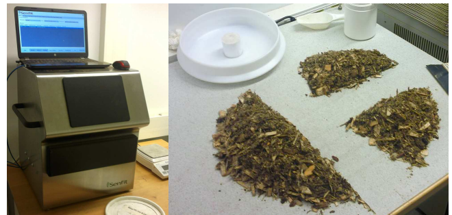
Fig. 2. Senfit BMA Desktop, the microwave moisture measurement instrument on the left and the plate-shaped measurement bowl of the instrument with a crushed and milled stump sample divided in three parts on the right.
