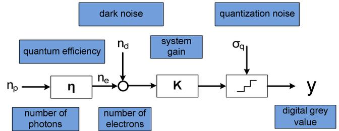
**Figure 3: Graphical representation of the system model [1]**
