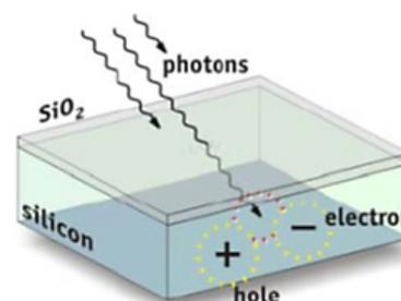
**Figure 1: Generation of electron-pairs inside the semiconductor [5]**
