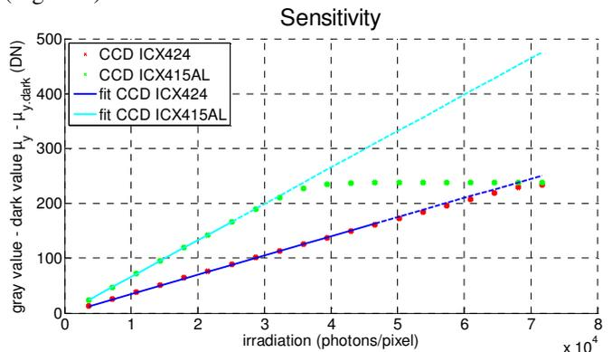
**Figure 7: Sensitivity measurements with different camera systems**
