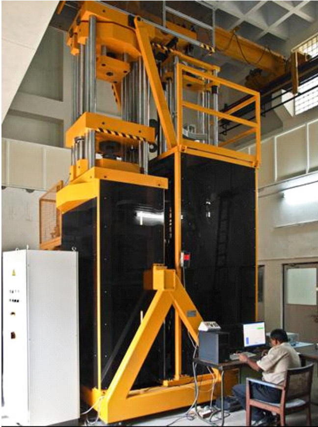
Fig. 2: A view of the 1 MN FSM installed at NPL(I)
