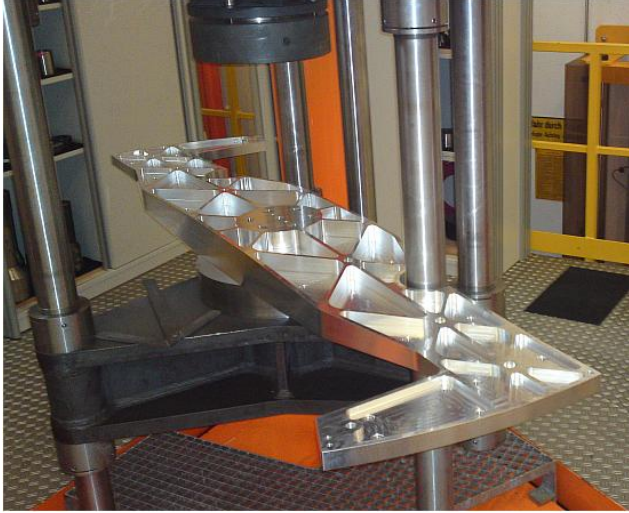
Fig. 6: The figure shows the first version of the aluminium lever mounted on the 1-MN force standard machine. The shown shape has been retained for the INVAR lever. One can also see the measurement points used to determine the position towards which the coordinate measuring machine later moves.
