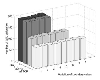
Figure 3: Variation of four boundary values and number of valid calibration without measurement noise, threshold value =  $50\mu m$
