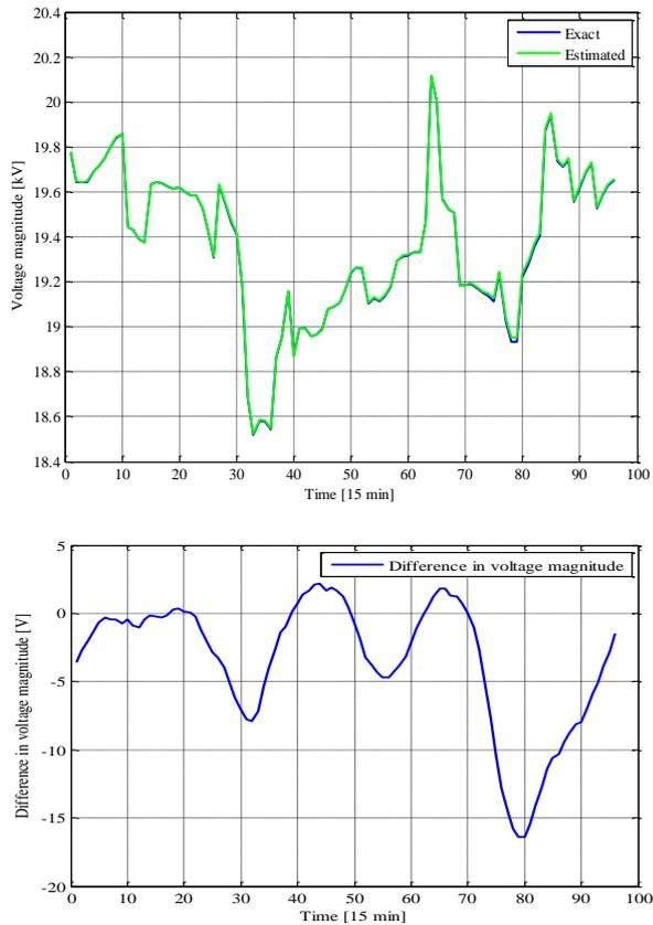
Figure 4: Actual and estimated voltage magnitude and difference between actual and estimated voltage magnitude at node no. 3.
