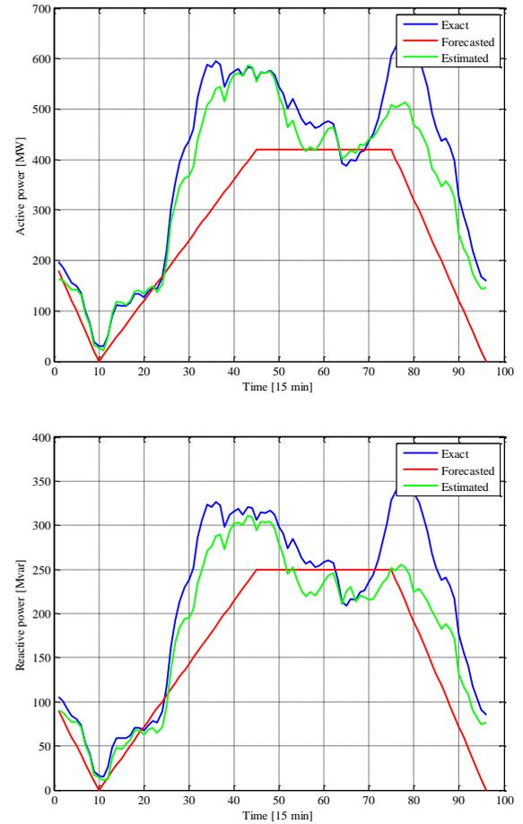
Figure 2: Results for node no. 3 with measurement of complex nodal voltages only at nodes no. 2, 4, 6 and 8, simple forecasts for all loads and given active and reactive power injection at node no. 2.
