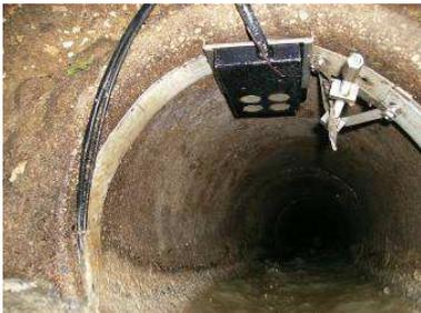
Figure 3. Flow measurement device: detail of ultrasound device (four pairs) for flow depth measurement
