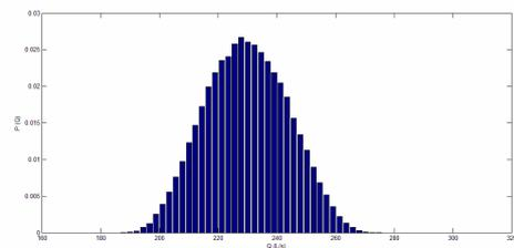
Figure 9. Flow rate output PDF for  $u(\beta) = \pm 1\%$
