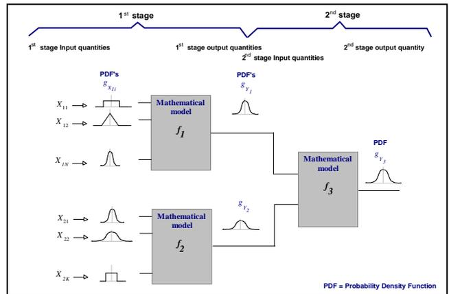
Figure 4. Propagation of density probability functions in a two stage measurement system
