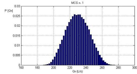
Figure 5. Output PDF of flow rate obtained for MCM n. 1
