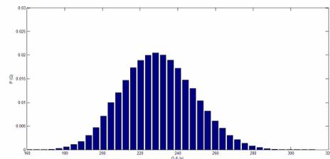
Figure 10. Flow rate output PDF for  $u(\beta) = \pm 5\%$
