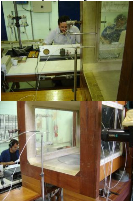
Fig. 3. Hot-wire anemometer (CTA) and static Pitot tube at the Wind Tunnel Test section of IPT.
