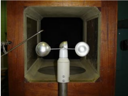
Fig. A3. Cup anemometer positioned at the discharge of the wind tunnel.
