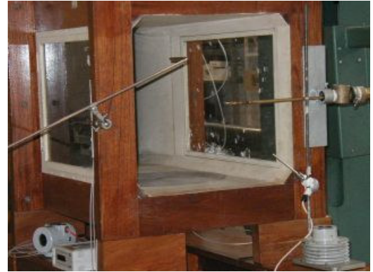
Fig. A6. A Cole Pitot tube calibrated in air.
