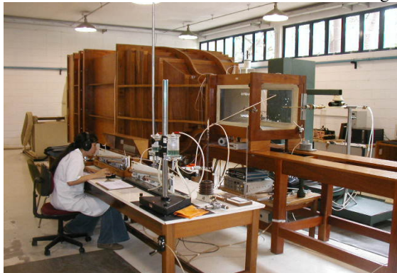
Fig. 1. Wind Tunnel of IPT for anemometer and Pitot tubes calibration.
