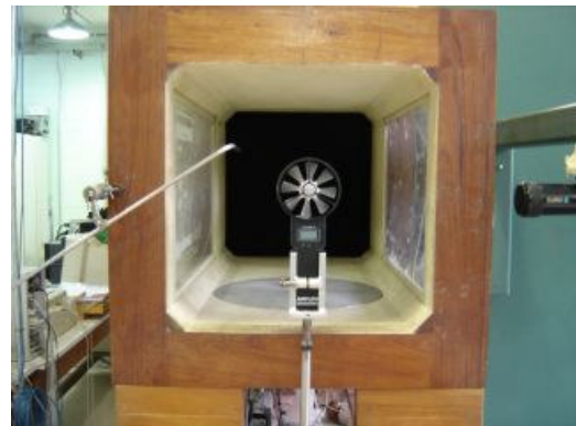
Fig. A1. Typical vane anemometer positioned at the wind tunnel test section.
