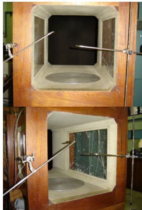
Fig. 2. Wind Tunnel Test section of IPT. Two static Pitot tube were used to measure the velocity profile.
