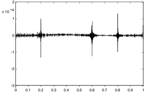
Fig.3. The dynamic error  $e(t)$  after correction
