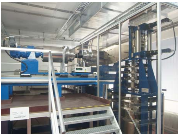
Fig. 1. View of one set of masses, lever and operation platform
