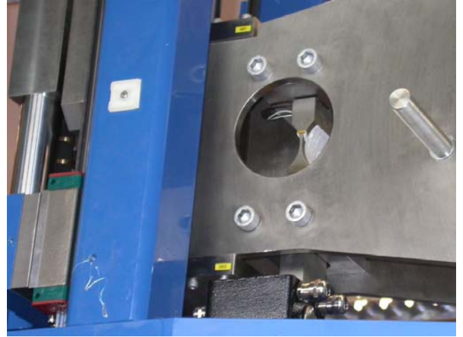
Fig. 2. Strain-controlled mass hinge
