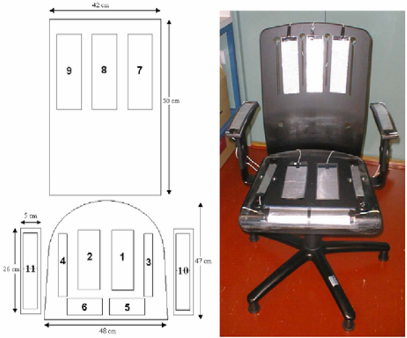
Fig. 2. EMFi sensors fixed on an office chair.
