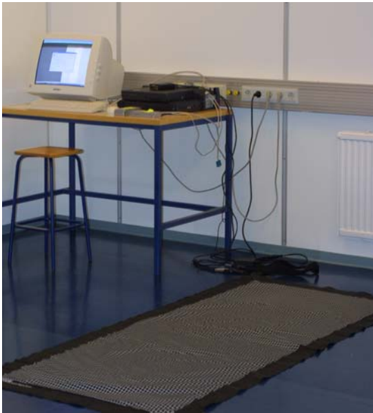
Fig. 3. The Xsensor system: sensor mat, laptop computer with Xsensor software and read-out electronics.
