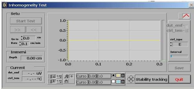
**Figure 3: User interface to the program for control of the hardware, data acquisition, analysis and storage.**
