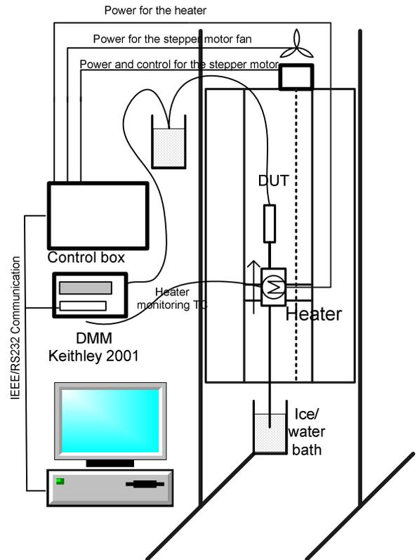
**Figure 2: Connection scheme of the Thermocouple inhomogeneity testing device when used in moving heater configuration.**
