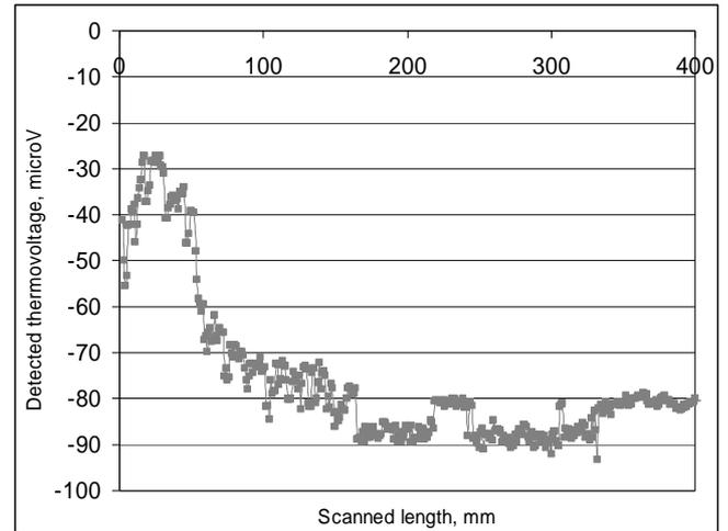
**Fig. 2. Measured emf during inhomogeneity test.**
