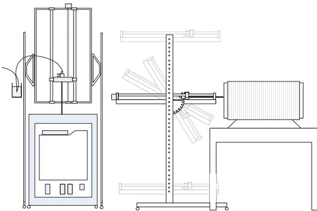
**Figure 1: Drawing of the frame of the Thermocouple Inhomogeneity Testing Device. On the left default configuration for immersion testing is shown. Frame can be tilted in six steps from vertical to horizontal, and adjustable space between legs allows to position device above baths and furnaces of different width.**
