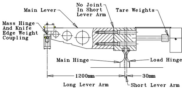
Fig. 2. Lever, lever support and weight coupling
