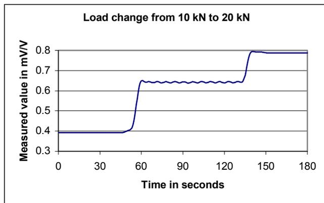
Fig. 5a. Typical load change sequence (deadweight machine)
