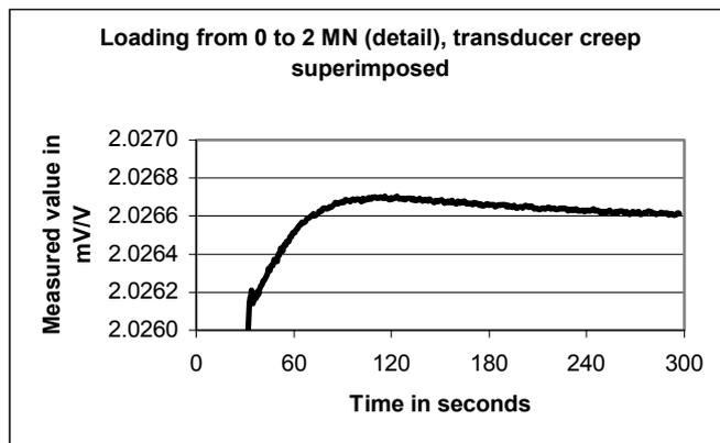
Fig. 5b. Typical load stability (lever machine)
