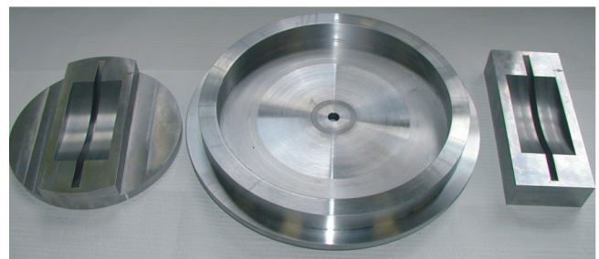
Fig. 3: Rotatable calibration body with bearing
