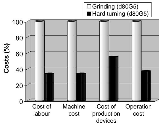
Fig. 14. Comparison of data of time (%) for grinding and hard turning in machining of gear's bore
