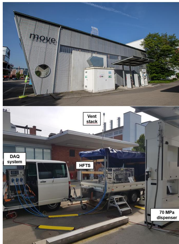
Figure 1: Top) General view of the Empa HRS, the hydrogen dispenser is at the extreme right, bottom) METAS gravimetric standard installed at the Empa HRS.
