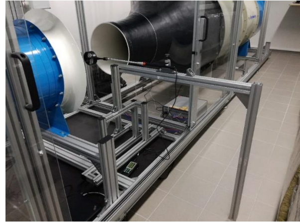
Figure 10: Construction for shifting the anemometers
