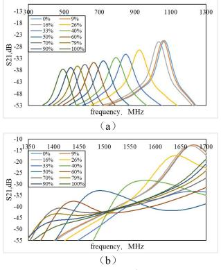
Figure 5:  $TM_{010}$  and  $TM_{110}$  mode response to water cut(a)  $TM_{010}$  (b)  $TM_{110}$ ..
