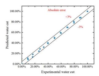
Figure 6: Predicted water cut VS experimental water cut.
