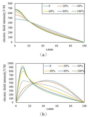
**Figure 3:** the Distribution of Electric Field Intensity(a) TM<sub>010</sub> (b) TM<sub>110</sub>.
