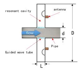
Figure 2: Microwave Resonant Cavity Sensor
