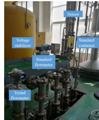
Figure 12: Diagram of the experimental verification set-up for electrode optimisation of electromagnetic flow meters.
