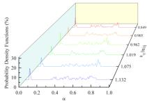
Figure 7: PDF distributions for slug flow ( $u_{sl}$  = 0.707 m/s)
