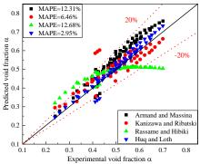
Figure 10: Measurement accuracy of stratified flow
