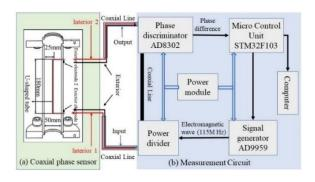
Figure.3. Coaxial line measurement system
