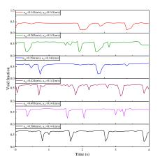
Figure 6: Void fraction time series of stratified flow ( $u_{sl} = 0.141 \text{ m/s}$ )
