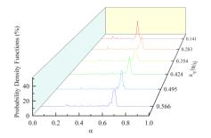
Figure 8: PDF distributions for stratified flow ( $u_{sl}$  = 0.141 m/s)
