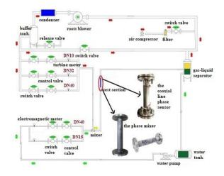
Figure 1: Experimental device diagram of coaxial line sensor.
