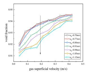
Figure 3: Relationship between gas superficial velocity and void fraction.
