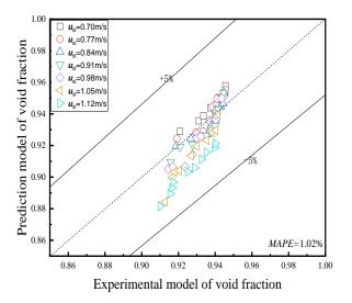
Figure 5: Comparison between experimental model of void fraction and optimized prediction model
