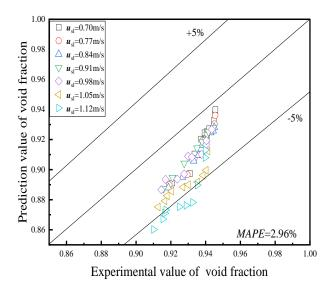
Figure 4: Comparison between experimental results and model prediction results
