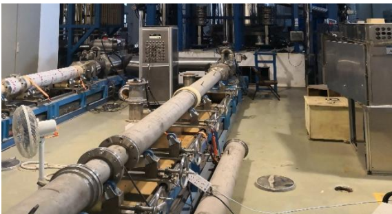
Figure 3: physical diagram of water flow standard device.
