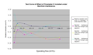
According to the above figure: ① Under the condition of manifold interference, the relative indication error curve trends of flowmeter C in the ideal flow state and at 30D and 20D of the upstream straight pipe segment are basically the same. The maximum change is not more than 0.21%. ②The relative error curve has different trends at 15D of the upstream straight pipe segment, with the maximum change up to 0.32%. ③Under manifold interference, when the operating
