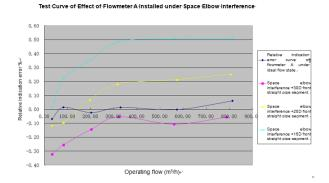
According to the above figure: (1) Under the condition of space elbow interference, the relative indication error curve trends of flowmeter A in the ideal flow state and at 30D and 20D of the
