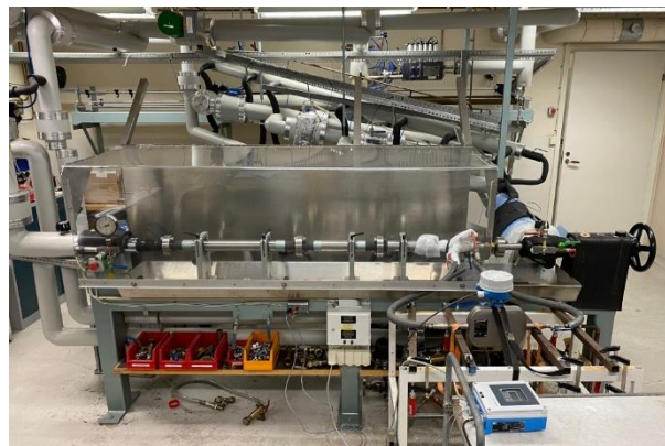
Figure 5: Calibration facility VM7 used for the measurements with water and temperatures between 10 °C and 30 °C.
