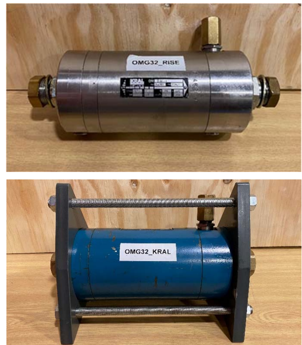
Figure 3: DUTs - top KRAL OMG-032 flow meter with stainless steel housing (Meter 1); bottom KRAL OMG-032 flow meter with carbon steel housing (Meter 2).
