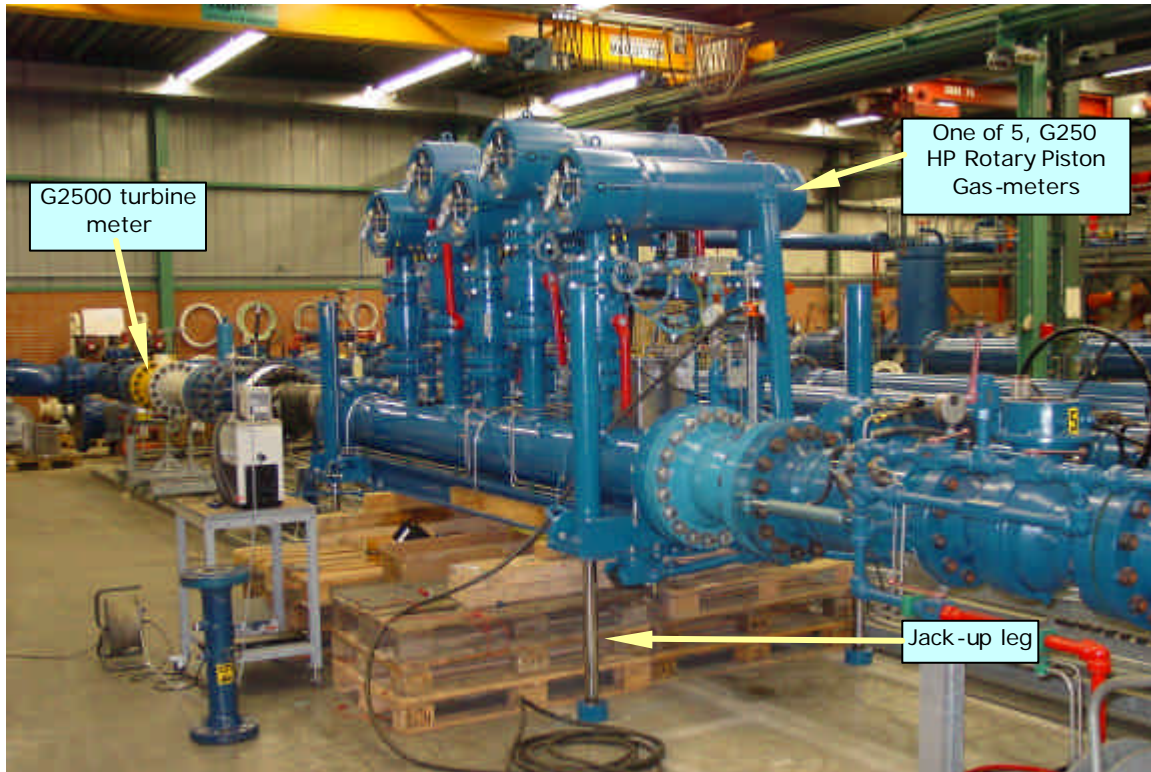
Figure 13 , Photograph of the setup in one of the meter runs of the "Bergum" facility
