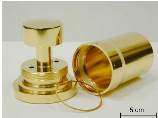
Fig. 5: LC resonator measurement cell
