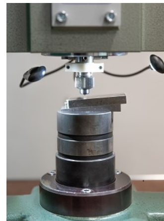
Figure 6: A study of alignment effects on GUM's Rockwell hardness standard machine
