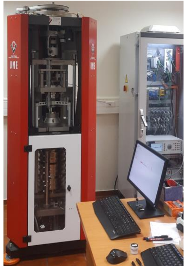
Figure 3: Rockwell-Brinell-Vickers Hardness Standard Machine of TÜBİTAK UME
