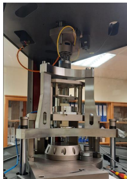
Figure 3: HLBHSM Force Application Mechanism; the force transducer and the frame
