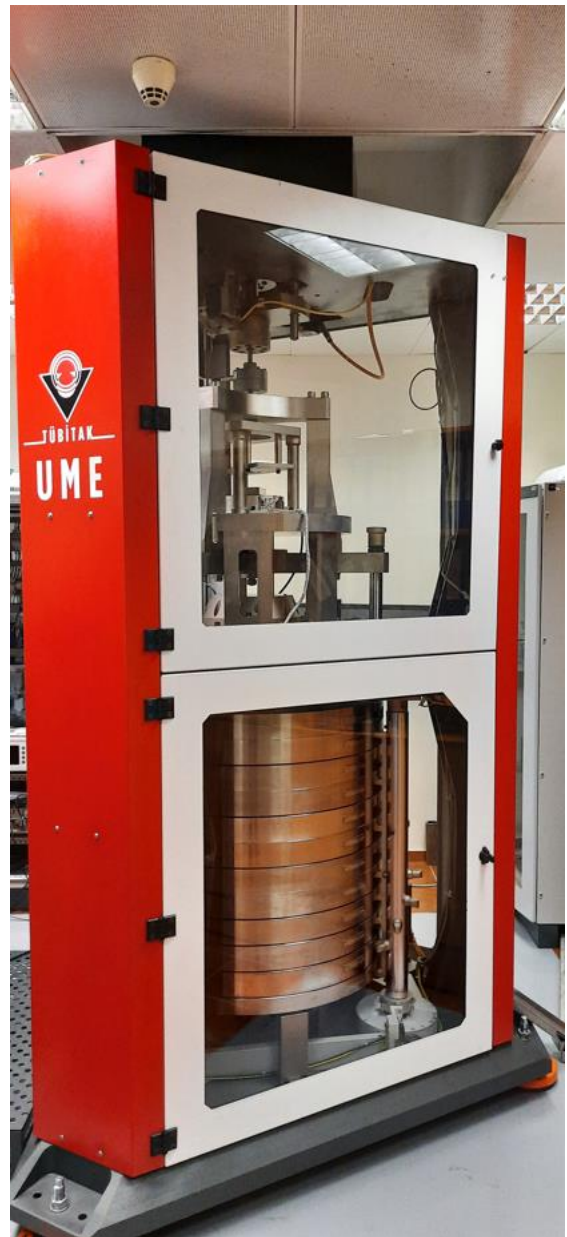
Figure 1: High Load Brinell Hardness Standard Machine of TÜBİTAK UME
