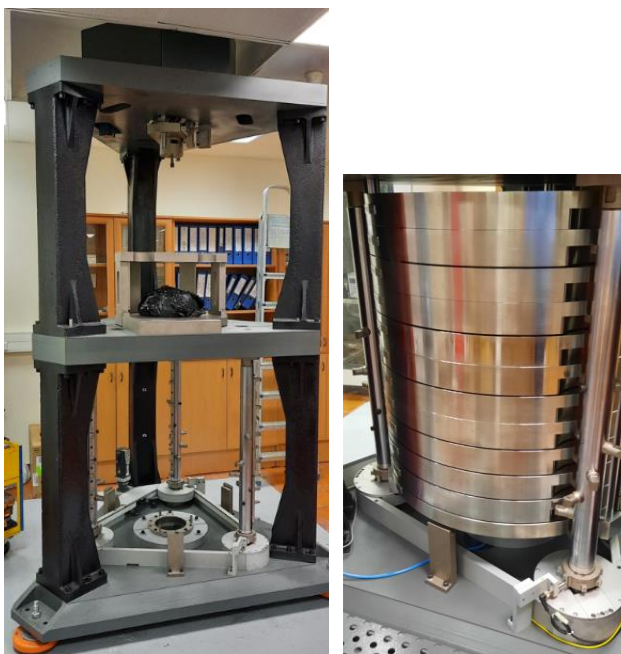
Figure 2: HLBHSM Body & Stainless Steel Mass Stacks
