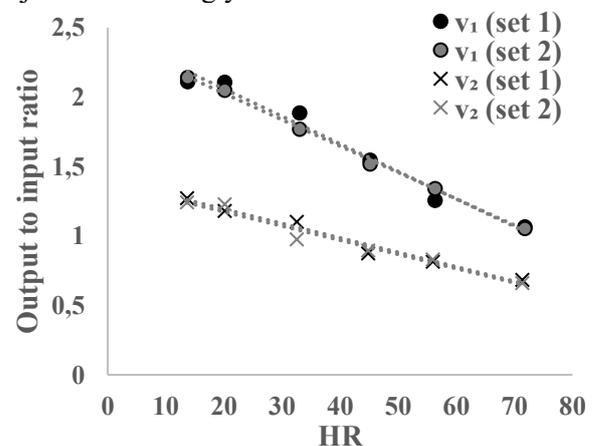
Figure 5: Linear relationship of the output to input ratio of velocities with respect to the measured hardness
