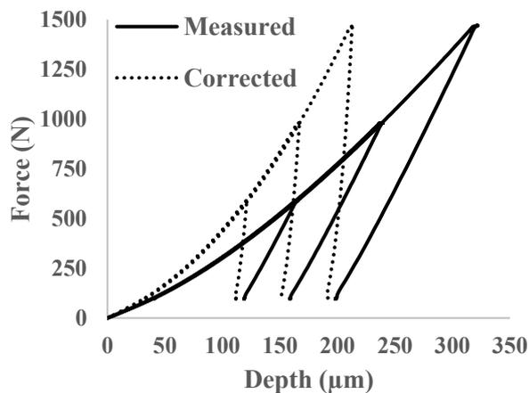
Figure 3: Load-displacement curves (HRA, HRD and HRC) before and after machine compliance correction
