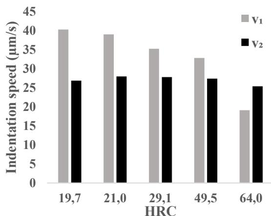
Figure 10: Measured indentation speeds for different hardness values
