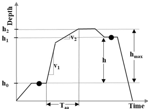
Figure 1: Typical indentation depth vs. time curve
