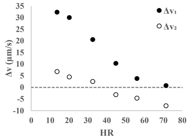
Figure 4: Variation of the difference between the measured and set velocity over the measured hardness
