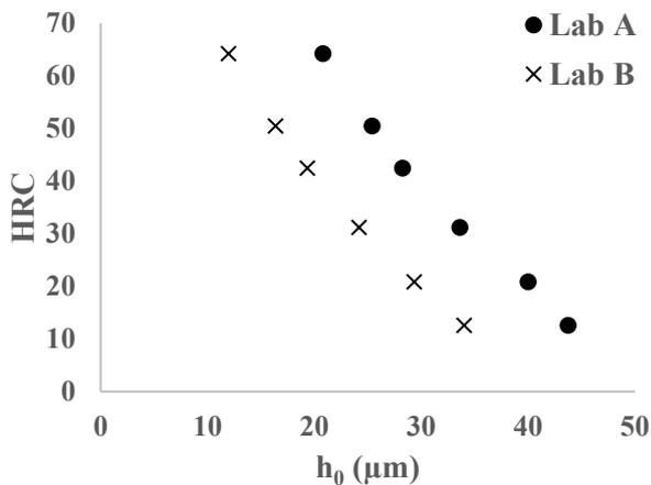
Figure 6: Machine-dependent characteristic curves (I)
