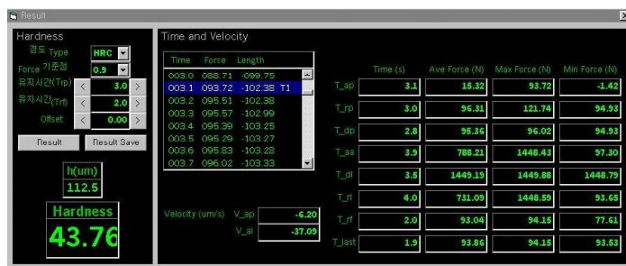
FIGURE 4. Photo of calibration results after a run of multi-calibration system for a testing cycle of Rockwell hardness
