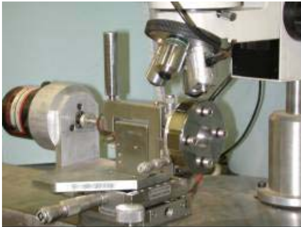
Figure 2 – Detail of the calibration of the angular encoder.
