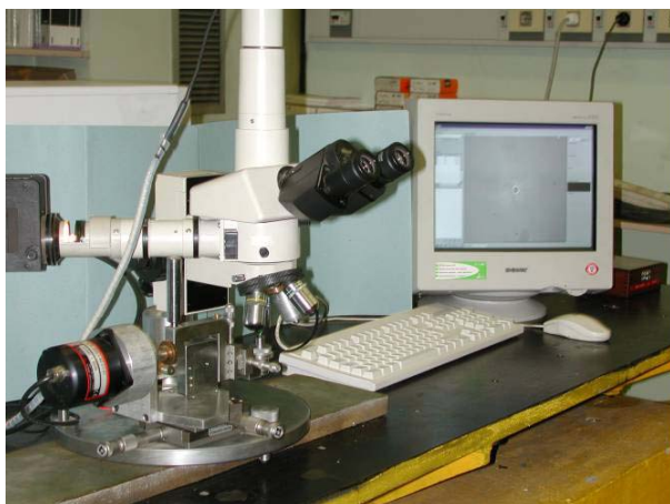
Figure 1 - Optical Measuring System for the calibration of the geometrical characteristics of diamond hardness indenters. The system is based on the interferometric image analysis of different sections of the indenters. It is composed of an optical microscope with interferometric lens, a rotating table for the indenters support (motorised by a DC motor and equipped with a calibrated angular encoder), a digital CCD camera and software specially developed for the analysis and measurement.
