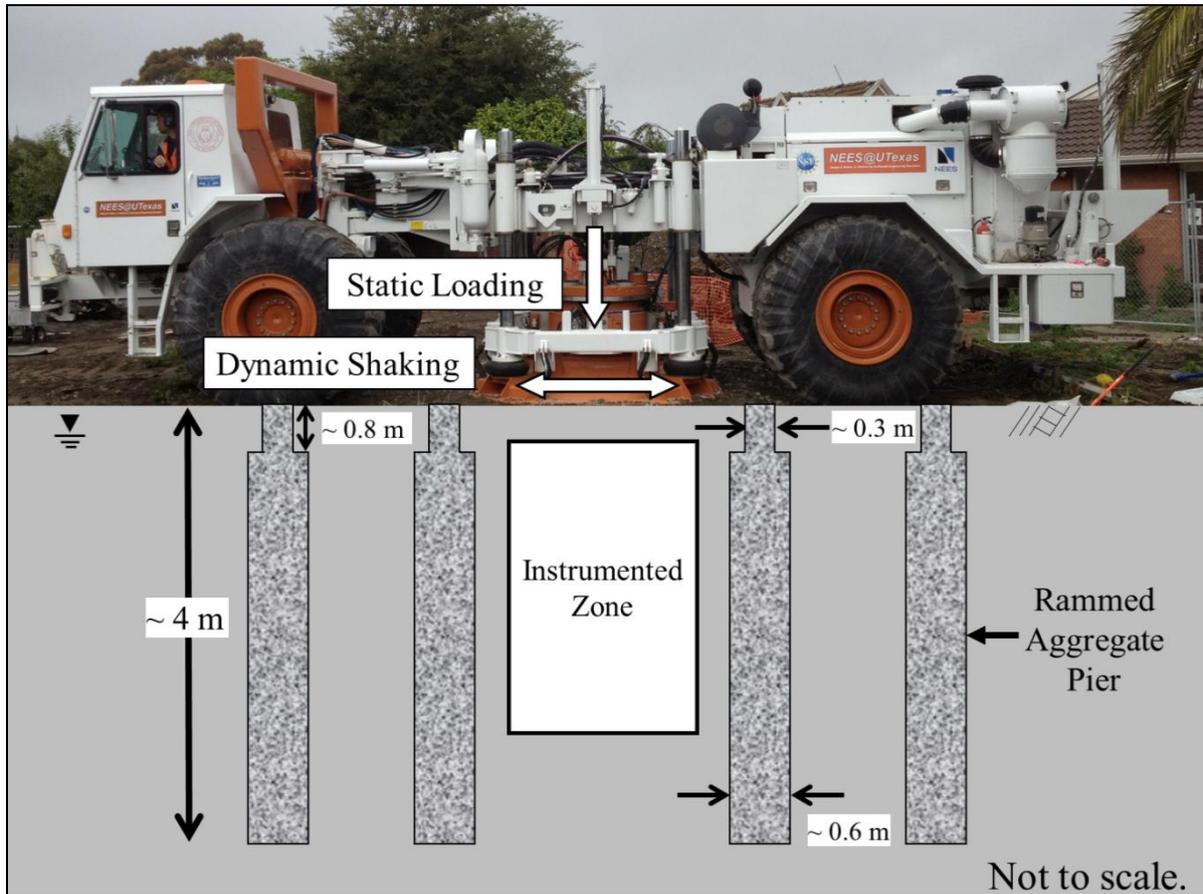
Figure 4: Cross-sectional perspective (Section A-A' in Figure 3d) of T-Rex in place to shake the RAP test panel.
