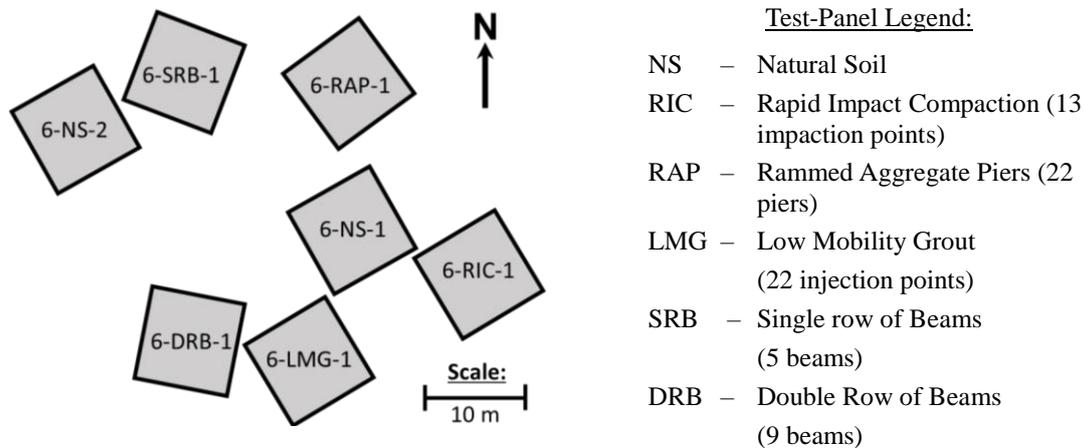
Figure 2: Test area at Site 6 with the relative locations of the seven test panels shown.
