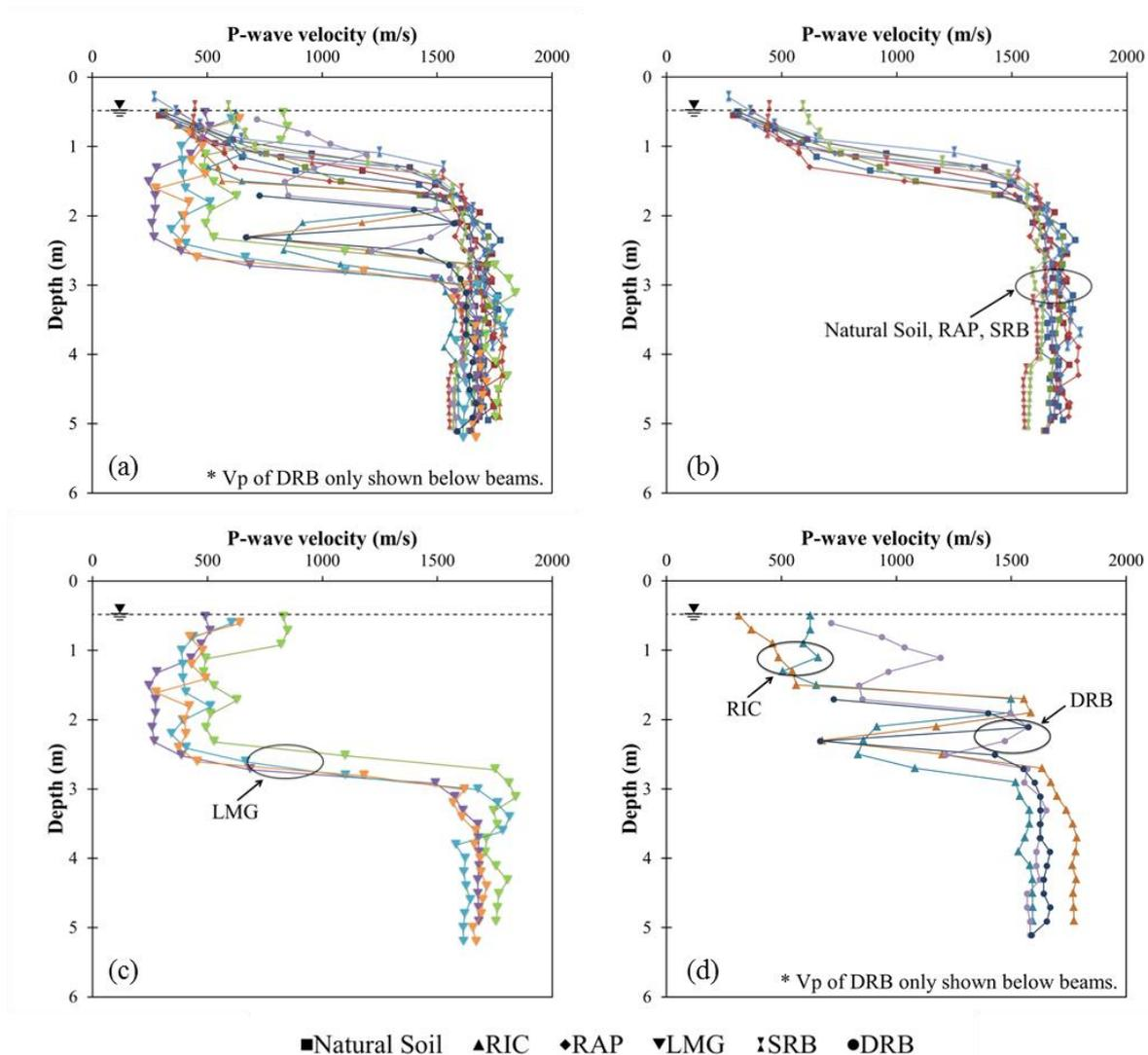
Figure 9: Profiles of compression (P) wave velocities at the seven test panels at Site 6: (a) two natural soil test panels, (b) between improvements at the RIC, RAP, SRB and LMG test panels, (c) across improvements at the SRB and DRB test panels and (d) across improvements at the RIC, RAP and LMG test panels.
