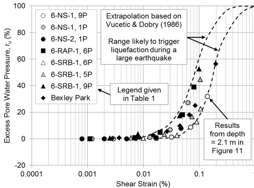
Figure 12: Compilation of T-Rex shaking results from five test panels that indicated soil liquefaction would likely be triggered in a large earthquake. (Note: The data for the 6-RAP-1 test panel is from a shallow depth of 1.15 m and likely results from the installation process loosening the shallow soil that had low confining stresses.)
