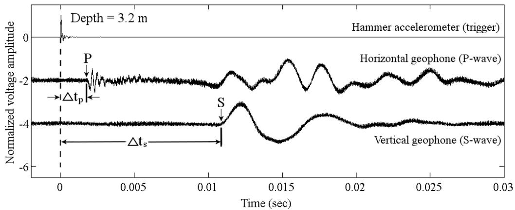
Figure 6: Travel-time records of compression (P) and shear (S) waves at one of the natural soil test panels at Site 6 (6-NS-1 in Figure 2). Example travel-time records with wave arrivals and associated corrected travel times in the soil are identified on the P and S waveforms. (Note: Relative location of crosshole testing is shown in Figure 3c.)
