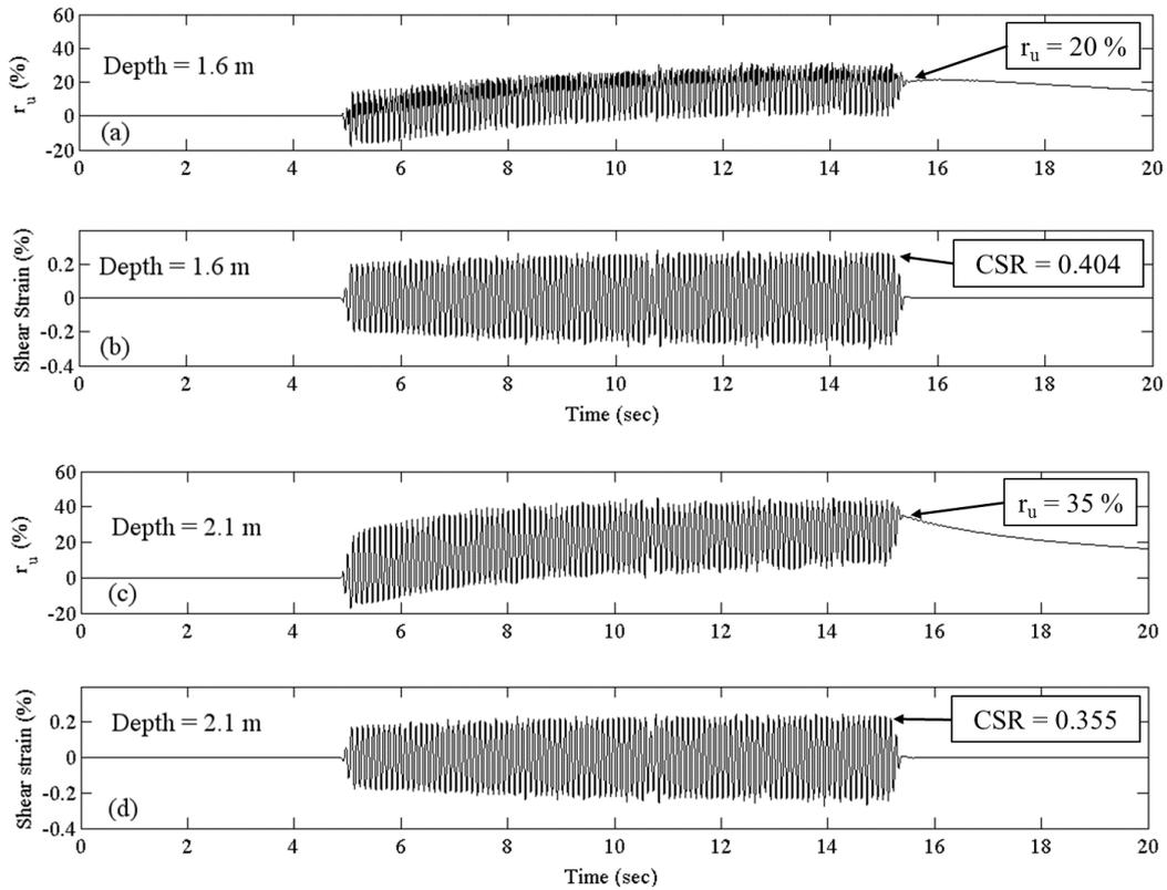
Figure 11: Variations of pore water pressure ratio,  $r_u$ , and shear,  $\gamma$ , strain with time determined from data recorded at the Natural Soil test panel (6 – NS-1) during T-Rex shaking at 10 Hz for 10 seconds; the final loading stage ( $\pm 107$  kN) and PPT depths of 1.6 and 2.1 m. (Note: The values of  $V_p$  and  $V_s$  at each depth are presented in Table 1.)
