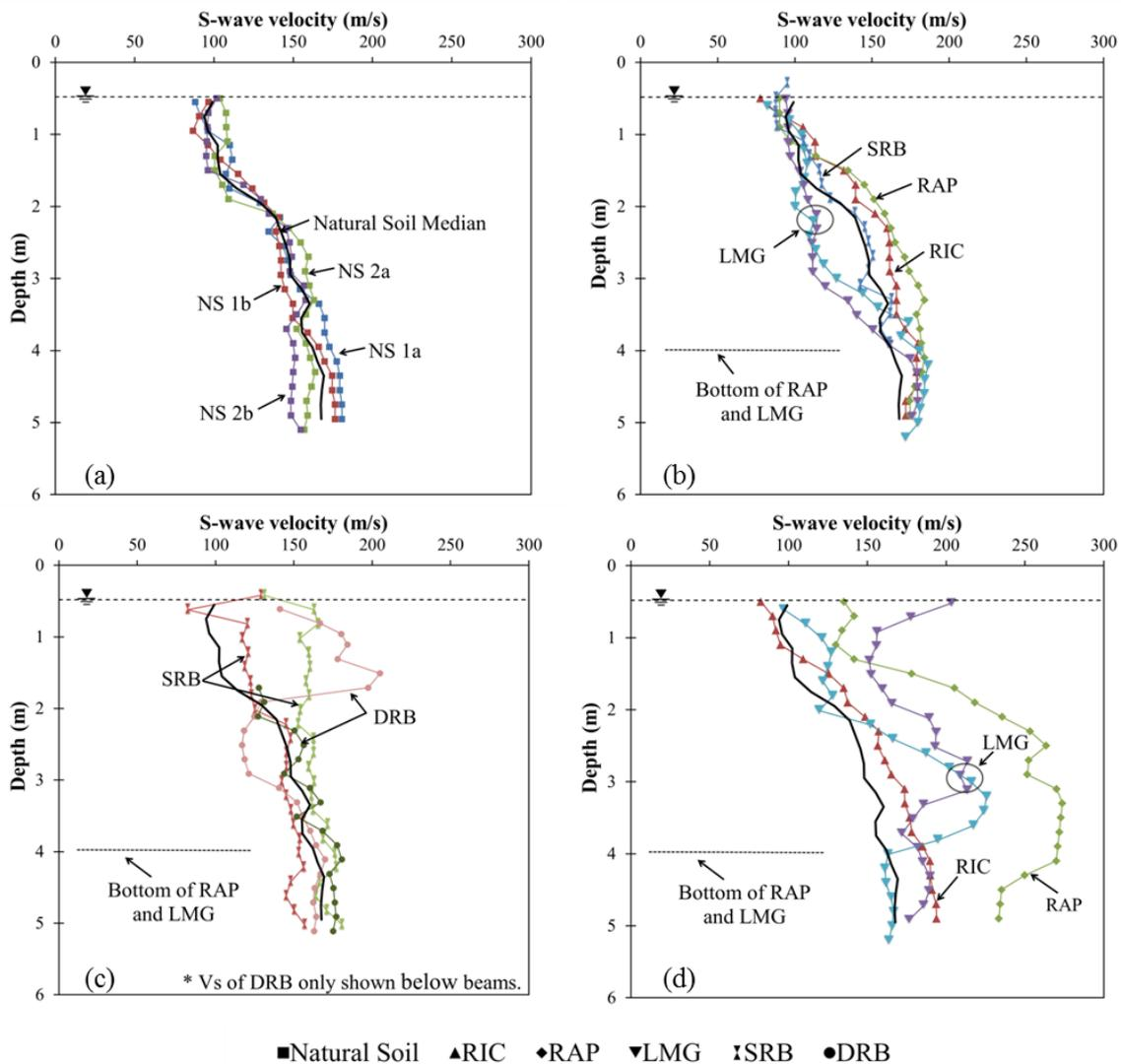
Figure 10: Profiles of shear (S) wave velocities at the seven test panels at Site 6: (a) two natural soil test panels, (b) between improvements at the RIC, RAP, SRB and LMG test panels, (c) across improvements at the SRB and DRB test panels and (d) across improvements at the RIC, RAP and LMG test panels.
