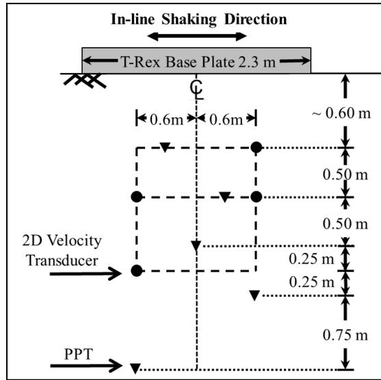
(b) Instrumentation array created in soil subsequently shaken by T-Rex; approximate locations projected on a vertical plane.
