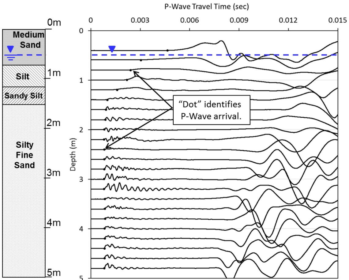
Figure 7: Complete set of P-wave, travel-time records measured at the 6-NS-1 test panel with the P-wave arrival identified on each waveform. (Note: All travel records have been corrected for travel time in the source rod.)
