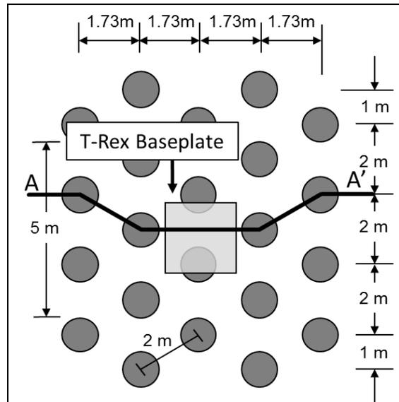
(d) Plan view showing the complete RAP test panel with 22 RAP columns, the location of the T-Rex baseplate, and cross-section A-A' used in Figure 4.
