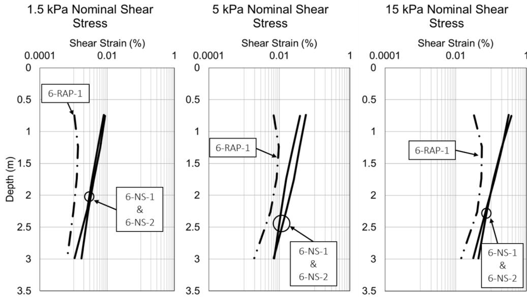
Figure 13: Relative stiffnesses of the RAP and natural soil test panels at Site 6 showing the stiffening effect of the RAP columns. Adapted from van Ballegooy et al. (2015a).
