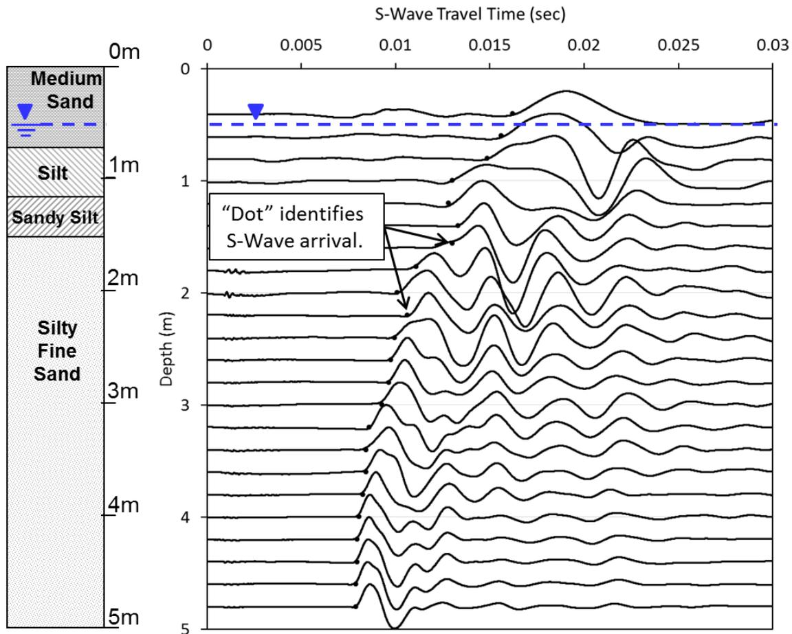
Figure 8: Complete set of S-wave, travel-time records measured at the 6-NS-1 test panel with the S-wave arrival identified on each waveform. (Note: All travel records have been corrected for travel time in the source rod.)
