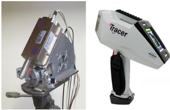
Fig. 1. XRF devices used for the experiments: F-70 (left) and Bruker Tracer 5g (right).
