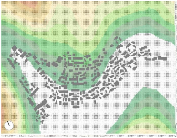
Fig. 4. Spatial model of Chuandixia (DEM and buildings) in the ENVI-met environment. Source: own elaboration.
