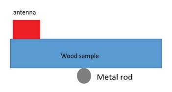
Fig. 2. GPR experimental setup
