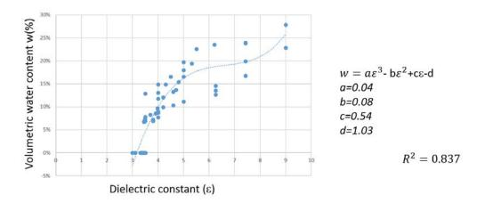
Fig. 4. Relationship between dielectric constant and volumetric water content
