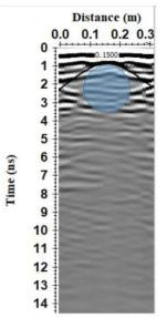
Fig. 3. GPR radar section with the diffraction curve analysis
