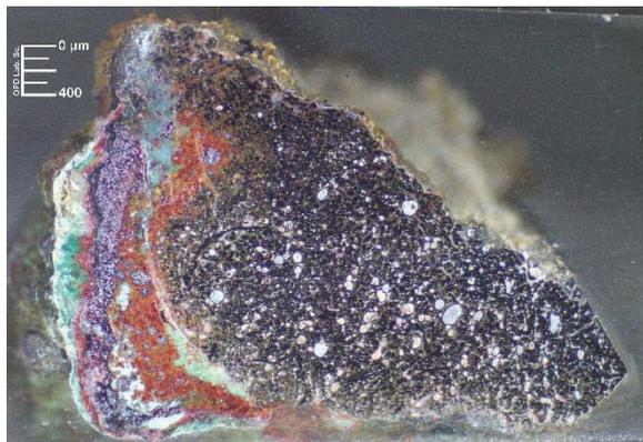
*Fig. 2. Dark field optical microscopy image of sample M1. As can be seen in the figure, the alloy fragment is deeply affected by mineralization phenomena that propagate from the surface to the bulk.*
