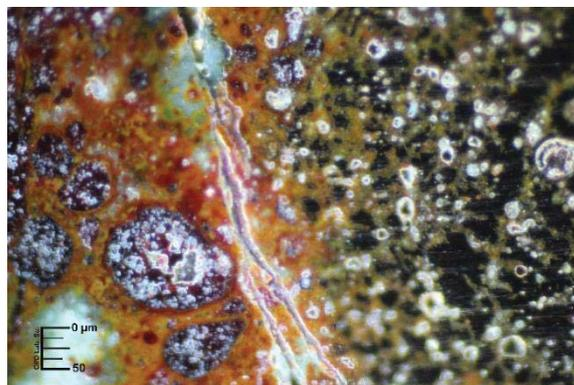
*Fig. 3. Dark field optical microscopy image of a detail of the M1 sample. The image shows how decuprification phenomena travel deep into the bulk of the metal, occupying porosities, cracks or interstitial space between the crystallographic grains. The tin-enriched decuprification areas appear orange due to the contribution of Pb and Sn oxides and cuprite.*
